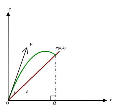
A projectile is fired from the origin with a velocity V and an angle of elevation  $\theta$ , where  $\theta \neq 90^\circ$ . You may assume that  $x = Vt \cos \theta$  and  $y = -\frac{1}{2}gt^2 + Vt \sin \theta$ , where x and y are the horizontal and vertical displacements of the projectile in metres from O at time t seconds after firing,
